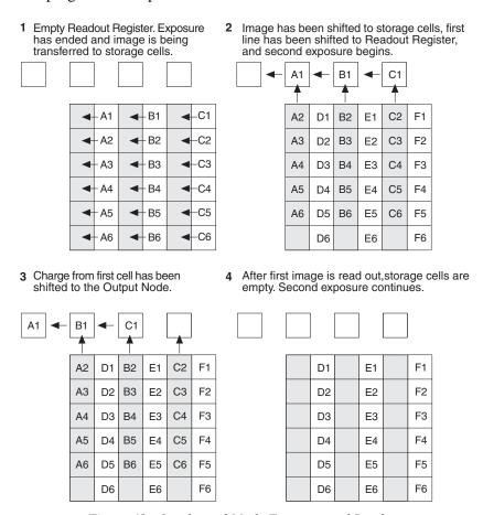
Figure 48. Overlapped Mode Exposure and Readout
